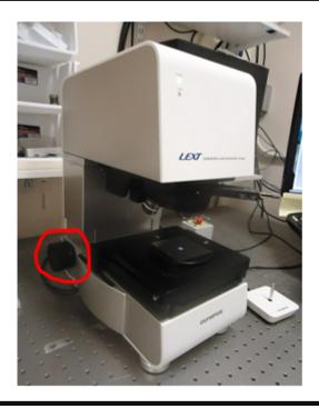
The blue dot shown on the sink surface shows that the microscope is on and ready to take a measurement.
