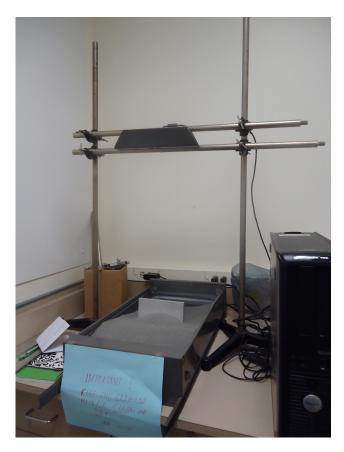
Figure 10 The sandbox with the Kinect at an adjusted height
