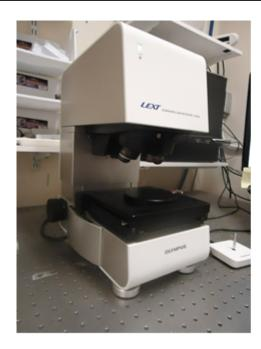
We are going to make a surface measurement using the Olympus LEXT microscope shown on the left.
