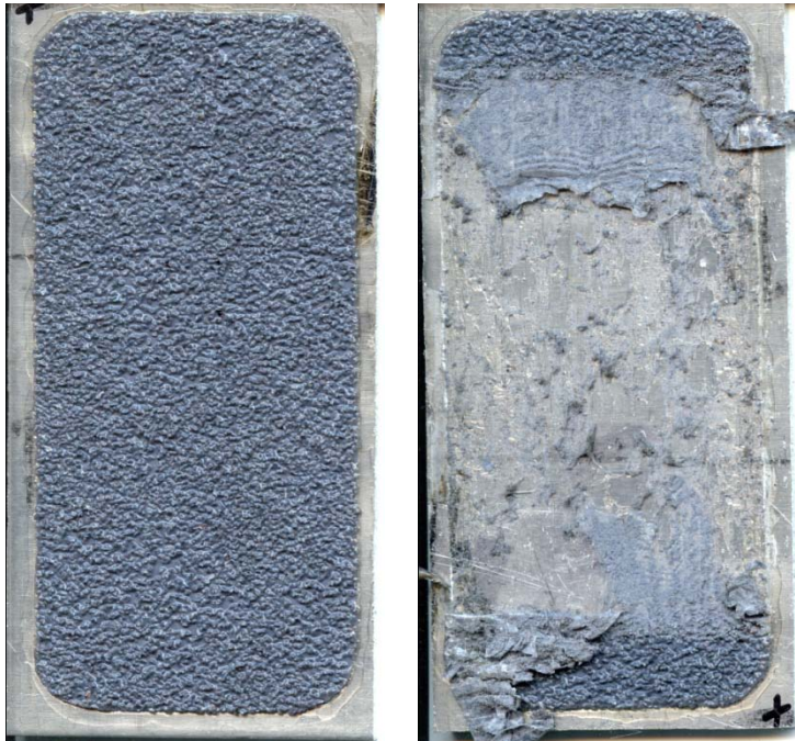
PNS 5456: Pre-Wear, 50 Cycles of Wear
