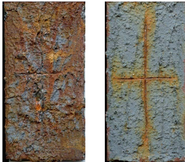
Figure 16: TNS A36 sample post corrosion testing, 1000 hours of salt fog chamber (left) and 864 hours On USCGC KODIAK ISLAND
