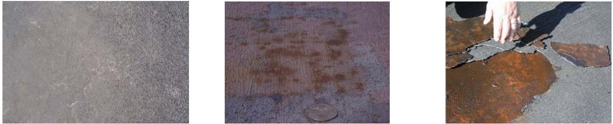
Figure 1: Traditional Non-Skid, Wear (left), Corrosion (middle), Failure (right) from: (Dust, 2008)
