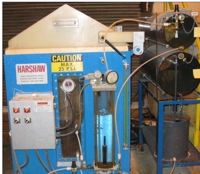
Figure 11: Salt Fog Testing Chamber at Ross Technology. Harshaw Environmental Chamber, Model 22, 3 Phase, 240 Volts, 60 Hz, 13 Amps. Made by Harshaw Chemical Co., Cleveland, Ohio.
