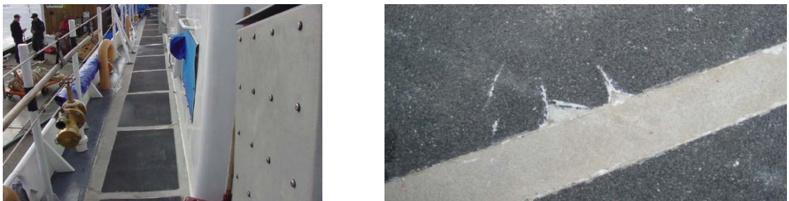
Figure 2: Peel and Stick Non-Skid, 110' Patrol Boat (left), Edge Failure (right) from: (Dust, 2007)
